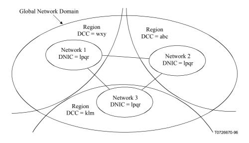
Figure H.3/X.121 – Global network composed of subnetwork identified by a common DNIC = 1pqr allocated from the global series
