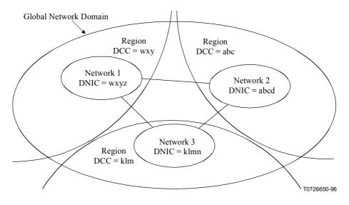
Figure H.1/X.121 – Global network composed of subnetworks identified by a DNIC appropriate to the region in which the subnetwork operates
