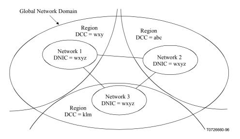
Figure H.2/X.121 – Global network composed of subnetworks identified by a common DNIC allocated to the parent network
