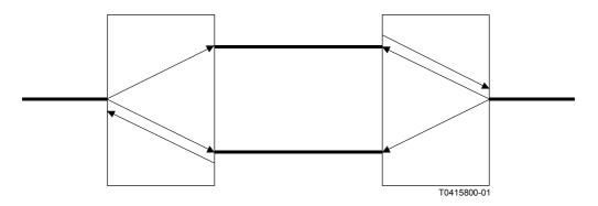
Figure 5/M.3100 – Configuration after roll operation in one NE
