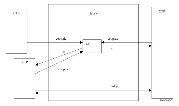
Figure 13/M.3100 – Roll operation (point-to-point unidirectional sink end)
