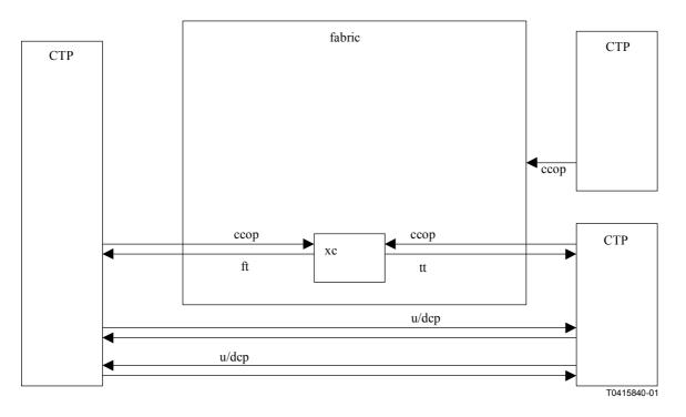
Figure 9/M.3100 – Release bridge operation (point-to-point bidirectional)
