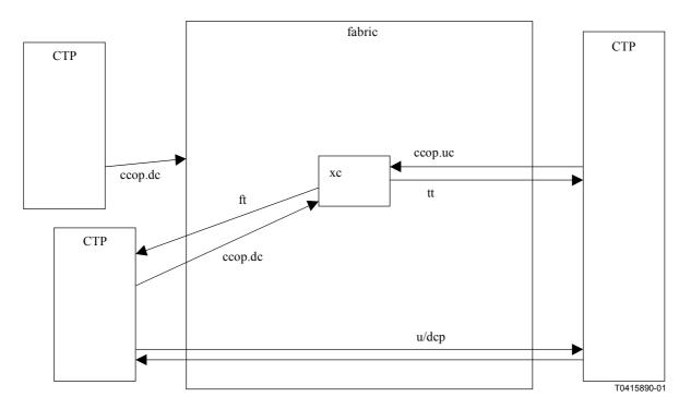
Figure 14/M.3100 – Release operation (point-to-point unidirectional sink end)
