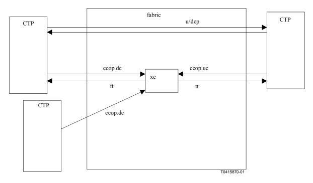
Figure 12/M.3100 – Bridge operation (point-to-point unidirectional sink end)
