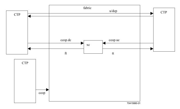
Figure 11/M.3100 – Initial configuration (point-to-point unidirectional sink end)
