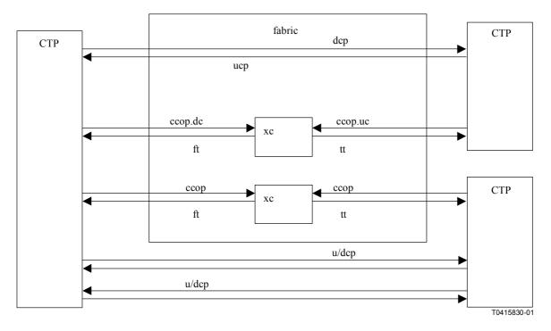
Figure 8/M.3100 – Roll operation (point-to-point bidirectional)
