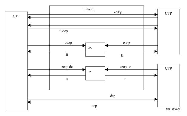
Figure 7/M.3100 – Bridge operation (point-to-point bidirectional)
