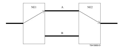
Figure 10/M.3100 – Unidirectional cross-connection
