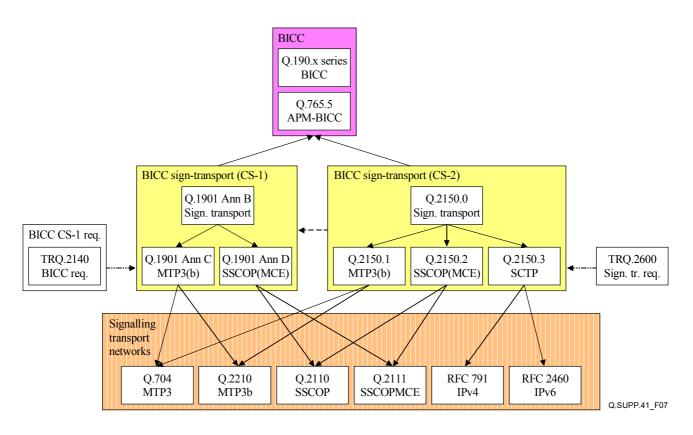
**Figure 7 – Signalling transport**
