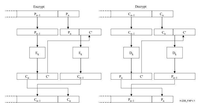
Figure I.1/H.235 – Ciphertext stealing in ECB mode
