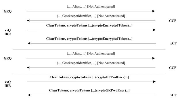
Figure B.2/H.235 – Password with symmetric encryption
