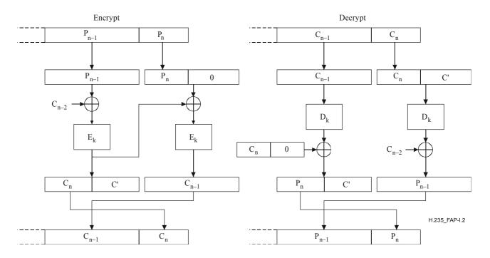
Figure I.2/H.235 – Ciphertext stealing in CBC mode
