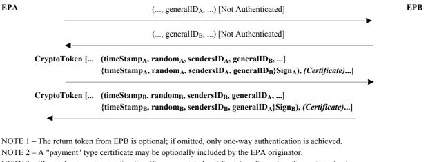
NOTE 3 – Sign indicates a signing function (from associated certificate) performed on the contained values.
