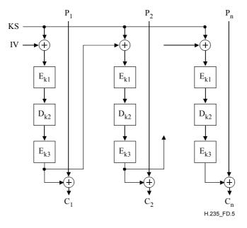
Figure D.5/H.235 – Triple-DES encryption in outer EOFB mode
