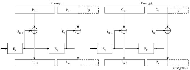
NOTE  $-S_i$  is the result of repetitive encryption (i.e. permutations) of the IV.
