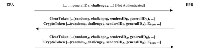
NOTE  $1 - challenge_A$  and the return encrypted **CryptoToken** from B to A are not necessary if one-way authentication is desired.
