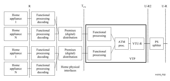
Figure 2/H.610 - VTP grouping which implements a fully distributed CPE approach
