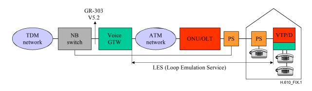
Figure IX.1/H.610 – VoDSL network elements
