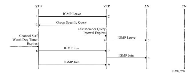
1 The end user is already watching a broadcast TV channel. He then selects another broadcast TV channel. The STB requests that the previously selected broadcast TV stream is disconnected. This is achieved by issuing an IGMP Leave containing the IP multicast address of the channel that is to be disconnected. In addition the STB starts a "Channel Surf Watch Dog Timer" to guard against unnecessary generation of IGMP Join
