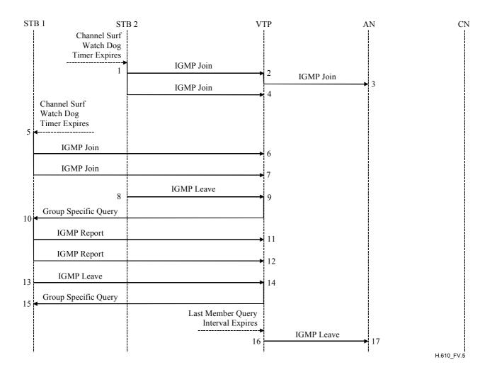
End user 2 selects a broadcast TV channel and the "Channel Surf Watch Dog" timer is started. Upon expiry of the "Channel Surf Watch Dog", STB 2 generates an IGMP Join specifying the multicast group address that the end user has selected. STB 2 also generates a second IGMP in order to cover the case the first one is lost (as specified by the robustness variable in RFC 2236).
