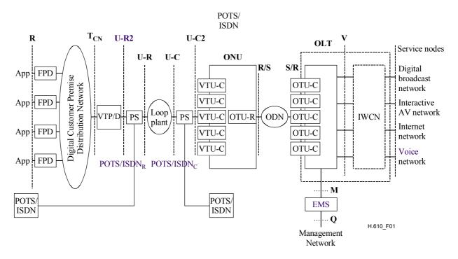
Figure 1/H.610 – FS-VDSL reference model
