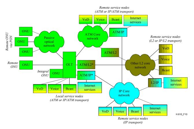
\* A local ATM/IP and/or ATM/L2 service node may be implemented in the same equipment as the OLT (the ATM interface becomes internal to the equipment).
