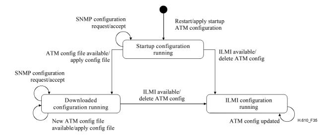
Figure 35/H.610 – State machine for the VTP/D ATM layer configuration
