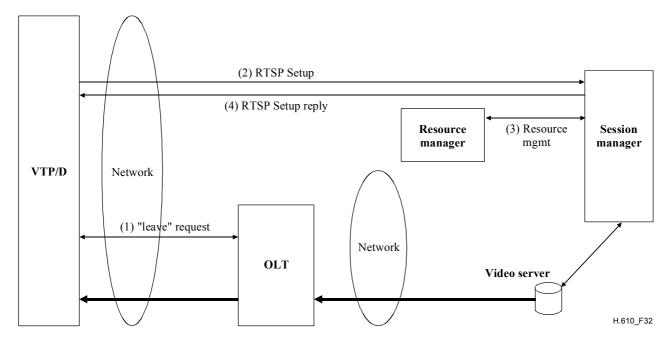
Figure 32/H.610 - VoD session establishment - Pre-established bandwidth end-to-end
