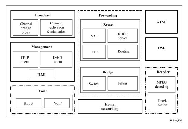
Figure 27/H.610 – VTP functional blocks
