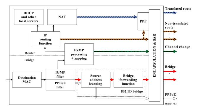
Figure I.1/H.610 – VTP upstream protocol processing
