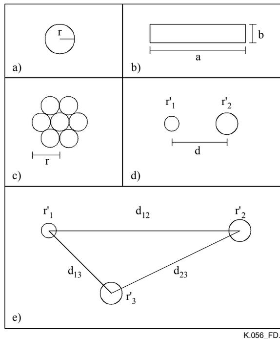
Figure D.1/K.56 – Geometric mean radius of typical conductors
