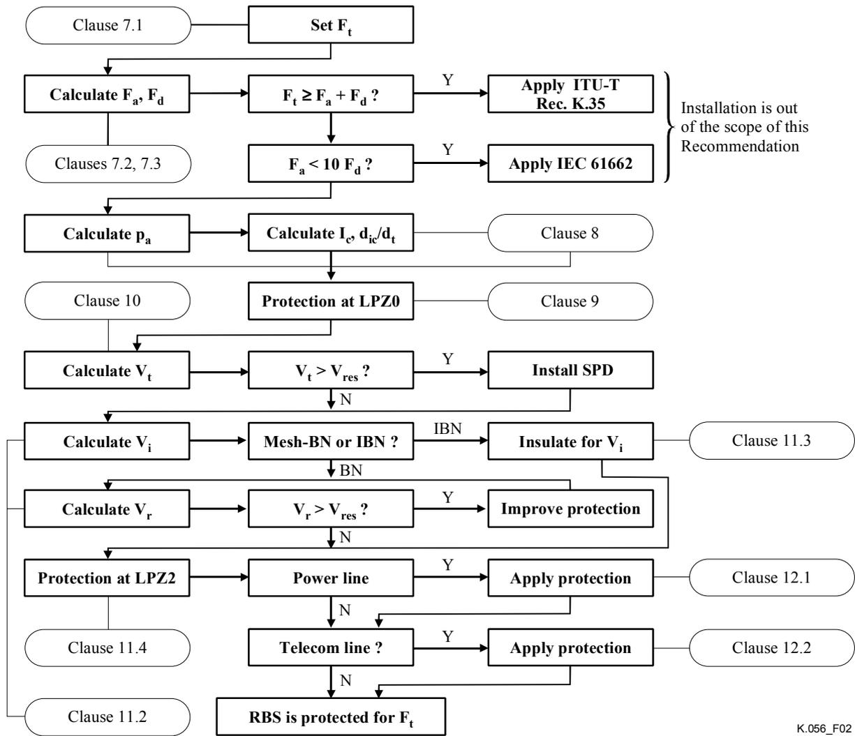
Figure 2/K.56 – Flow diagram for protecting a RBS against lightning
