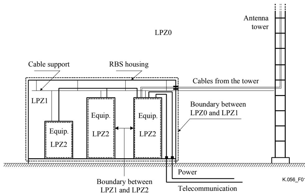
**Figure 1/K.56 – Reference configuration for a RBS**
