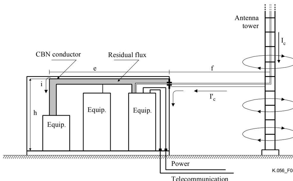
**Figure 4/K.56 – RBS with Mesh-BN configuration**
