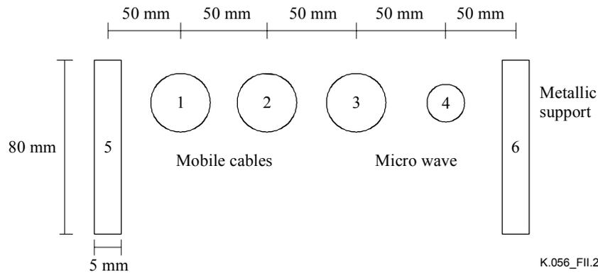
**Figure II.2/K.56 – Bundle off conductors along the tower (cross section view)**
