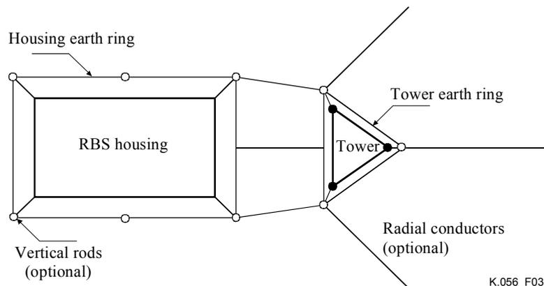
**Figure 3/K.56 – Earth configuration for the RBS**
