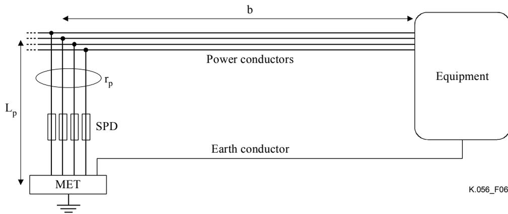
**Figure 6/K.56 – Assessment of the maximum length between power conductors and MET**
