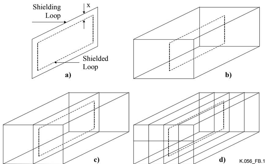
**Figure B.1/K.56 – Typical shielding configuration for RBS**
