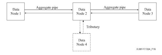
Figure 16/X.87/Y.1324 – A MSR topology, link-type with adding and dropping tributary services
