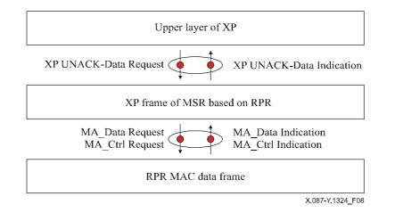
Figure 8/X.87/Y.1324 – Relationship between XP and RPR MAC, upper layer and XP
