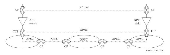
Figure 3a/X.87/Y.1324 – XP layer network example
