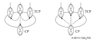
Figure 5/X.87/Y.1324 – XP layer multipoint connection points examples
