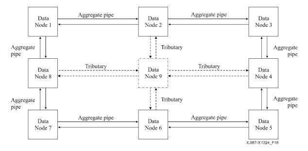
Figure 18/X.87/Y.1324 - A MSR topology, pseudo-mesh connection
