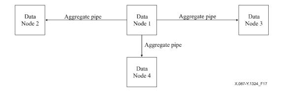
Figure 17/X.87/Y.1324 – A MSR topology, broadcast connection to DVB application
