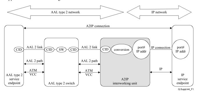
Figure 1 – Scope and definition of terms used in AAL type 2 to IP signalling interworking
