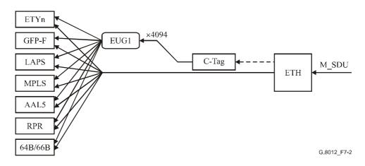
Figure 7-2/G.8012/Y.1308 – Ethernet single level multiplexing
