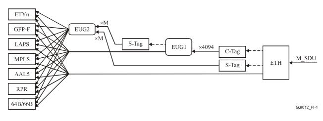
Figure I.1/G.8012/Y.1308 – Ethernet two-level multiplexing
