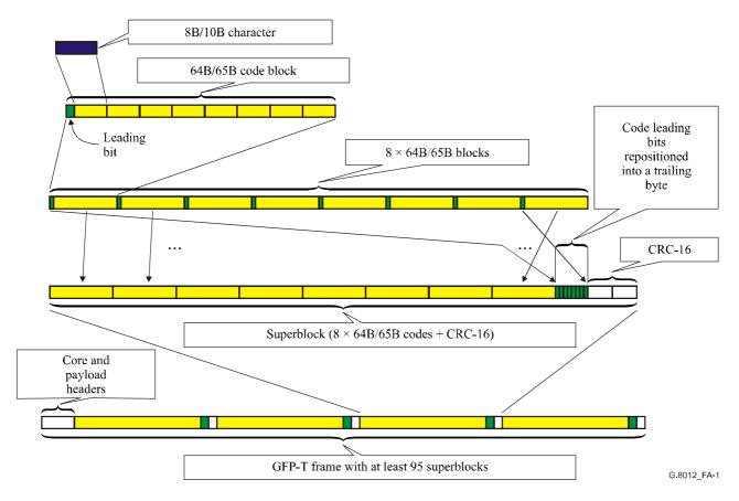
Figure A.1/G.8012/Y.1308 – GFP-T mapping for 8B/10B encoded 1 Gbit/s Ethernet
