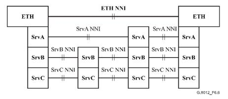
Figure 6-6/G.8012/Y.1308 – Example of layer networks in Ethernet NNI for case of interconnecting two ETH layer service nodes
