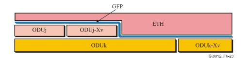
Figure 6-23/G.8012/Y.1308 – Components of the Ethernet over OTH NNI
