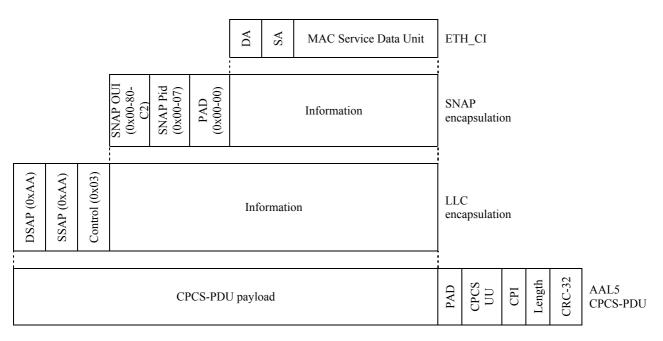
Figure 6-15/G.8012/Y.1308 – LLC encapsulation based AAL5 CPCS-PDU link frame without MAC FCS preservation
