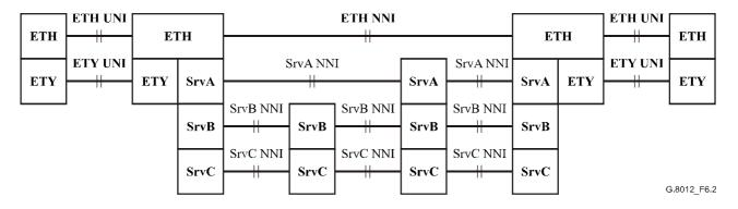
Figure 6-2/G.8012/Y.1308 – Example of layer networks in Ethernet UNI and NNI for case of pt-pt ETH layer connection
