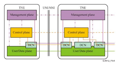
Figure 6-8/G.8012/Y.1308 – Three planes of Ethernet UNI and NNI
