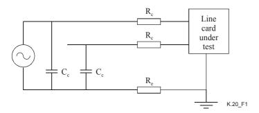
Coupling resistors  $R_{\rm e}$  represent the line resistances,  $C_{\rm e}$  represent the line capacitances to earth and  $R_{\rm e}$  represents the earthing resistance of the overvoltage protectors at the subscriber end of the line.
