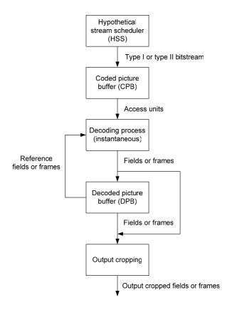
Figure C-2 – HRD buffer model
