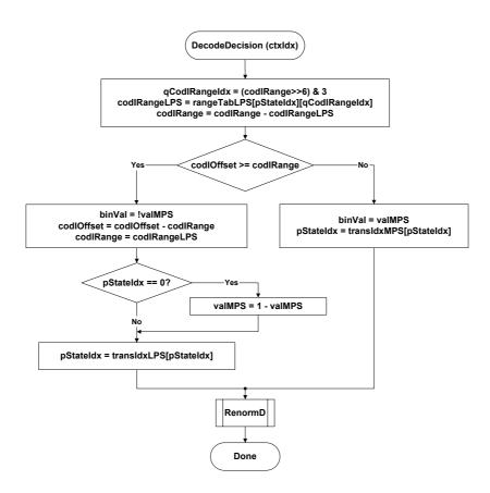
Figure 9-3 – Flowchart for decoding a decision
