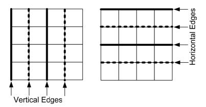
Figure 8-10 – Boundaries in a macroblock to be filtered
