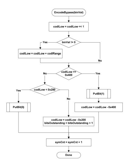
Figure 9-10 – Flowchart of encoding bypass
