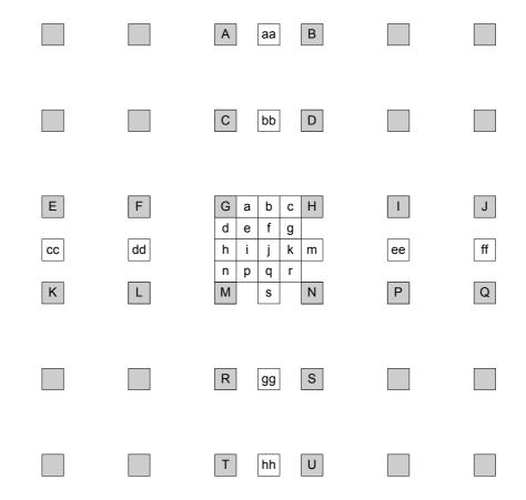
Figure 8-4 – Integer samples (shaded blocks with upper-case letters) and fractional sample positions (un-shaded blocks with lower-case letters) for quarter sample luma interpolation
