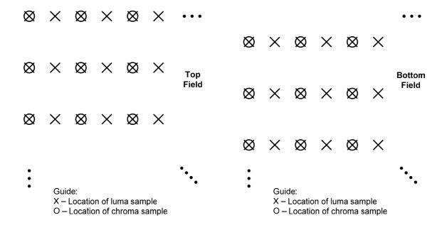
Figure 6-4 – Nominal vertical and horizontal sampling locations of 4:2:2 samples top and bottom fields
