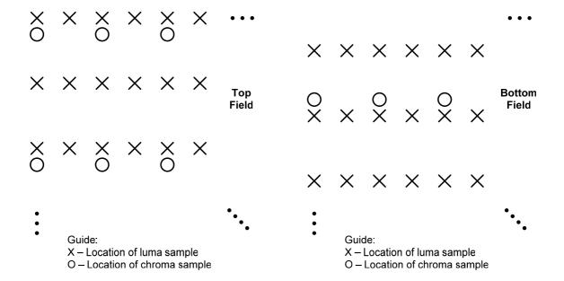
Figure 6-2 – Nominal vertical and horizontal sampling locations of 4:2:0 samples in top and bottom fields
