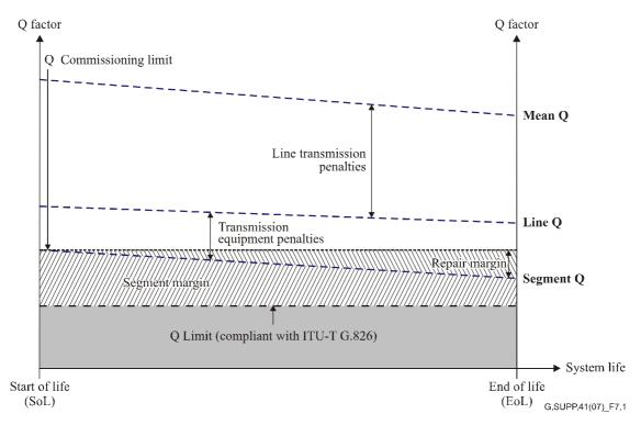
Figure 7-1 – Power budget structure example
