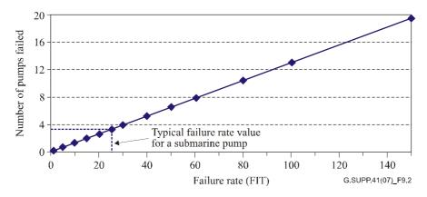
Figure 9-2 – Estimated number of pump failed in the 25 years for a typical transatlantic link composed of 1 fibre pair and 150 repeaters containing four pumps each
