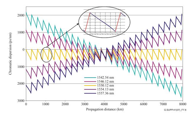
Figure 7-8 – Typical chromatic dispersion map for a submarine WDM system with 163 spans designed for 40 wavelengths centred around 1550.12 nm WDM system
