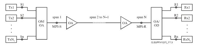
Figure 7-3 – Representation of optical line system interfaces (a multichannel N-span system)
