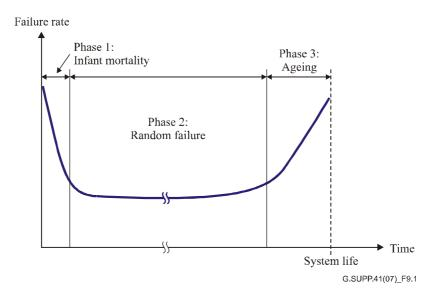
Figure 9-1 – Typical failure's rate behaviour during the life of a system
