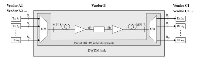
Figure 11-7 – Multi-span black-link transverse compatibility
