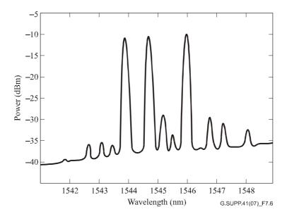
Figure 7-6 – Optical power spectrum measured at the output of 25 km length of dispersion shifted ( $D = -0.2 \text{ ps/nm} \cdot \text{km}$  at the central channel) when 3 mW channels are used [b-Tkach]
