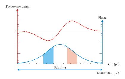
Figure 7-5 – Temporal variation of the phase shift and the frequency chirp induced by SPM [b-Agrawal]
