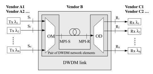
Figure 11-6 – Single-span black-link transverse compatibility
