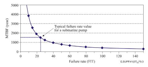
Figure 9-3 – MTBF for a second pump failure in the same repeater in a typical transatlantic link composed by 1 fibre pair and 150 repeaters with four redundant pumps each
