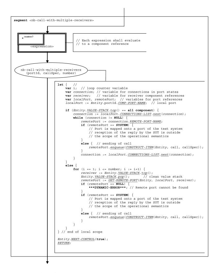
Figure 49-a – Flow graph segment <nb-call-with-multiple-receivers>
