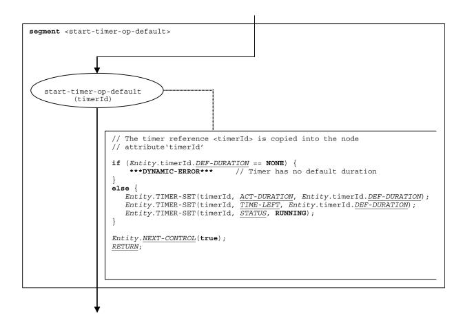
Figure 123 – Flow graph segment <start-timer-op-default>
