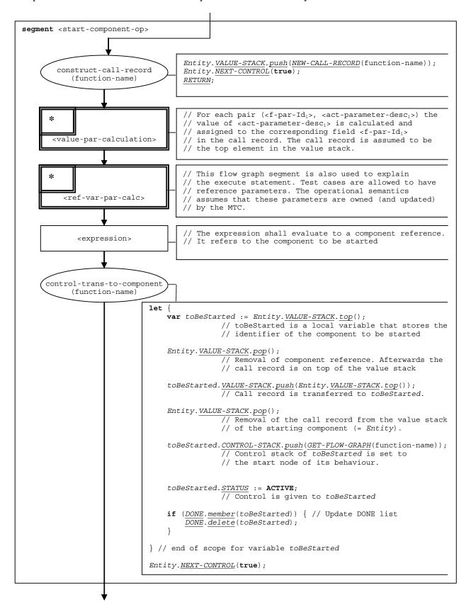
Figure 120 – Flow graph segment <start-component-op>
