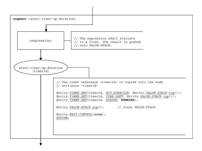
Figure 124 – Flow graph segment <start-timer-op-duration>
