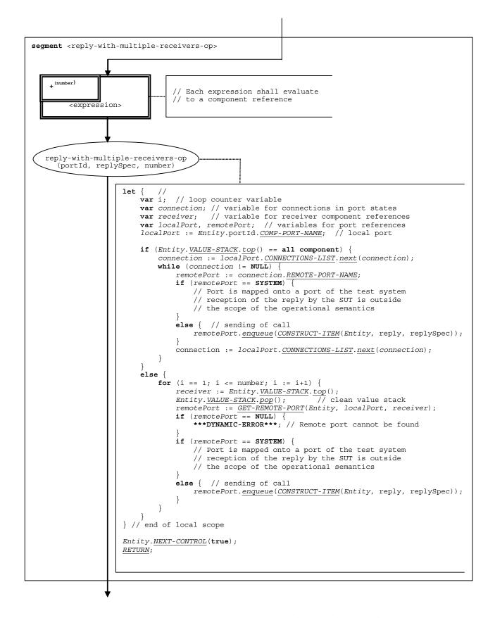
Figure 106-a – Flow graph segment <reply-with-multiple-receivers-op>
