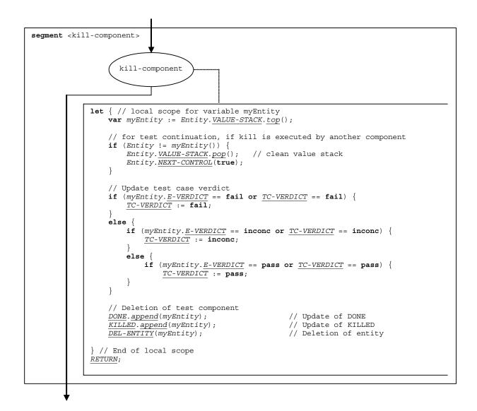
Figure 90-c – Flow graph segment <kill-component>
