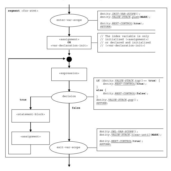
Figure 79 – Flow graph segment <for-stmt>
