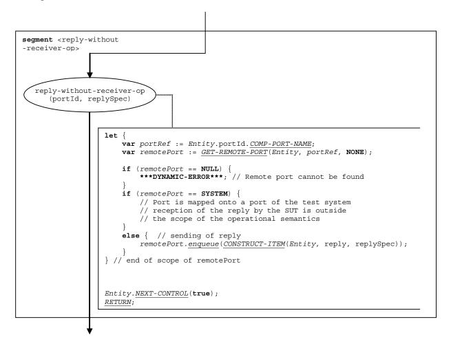
Figure 107 – Flow graph segment <reply-without-receiver-op>
