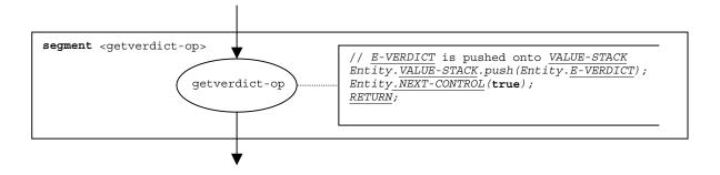
Figure 88 – Flow graph segment <getverdict-op>
