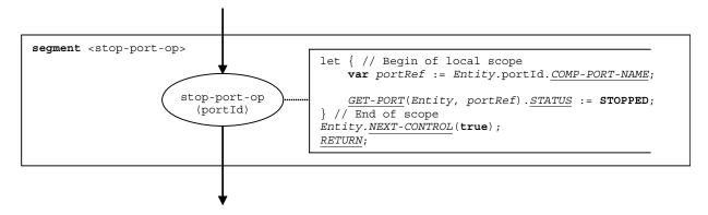
Figure 129 – Flow graph segment <stop-port-op>
