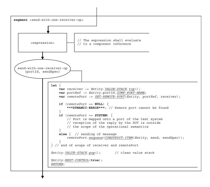
Figure 117 – Flow graph segment < send-with-one-receiver-op>
