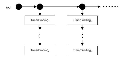
Figure 27 – Structure of the <u>TIMER-STATE</u> part of an entity state
