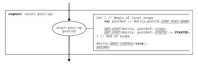
Figure 121 – Flow graph segment <start-port-op>
