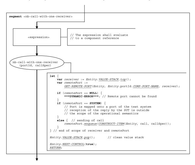
Figure 49 – Flow graph segment <nb-call-with-one-receiver>
