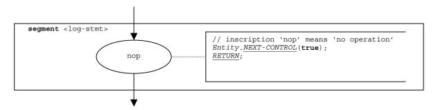
Figure 92 – Flow graph segment <log-stmt>
