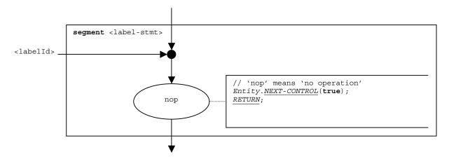
Figure 91 – Flow graph segment < label-stmt>
