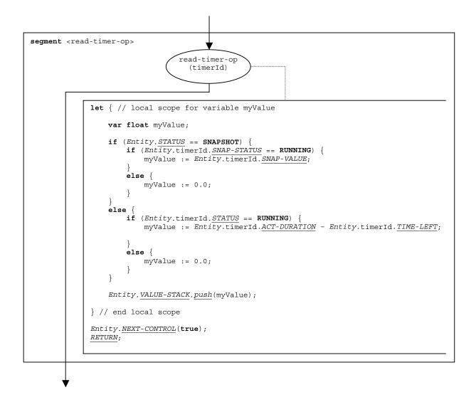
Figure 99 – Flow graph segment <read-timer-op>
