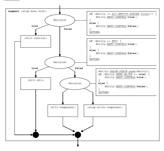
Figure 128 – Flow graph segment <stop-exec-stmt>
