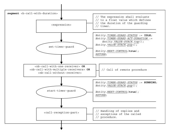
Figure 52 – Flow graph segment <b-call-with-duration>
