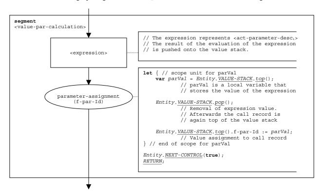
Figure 81 – Flow graph segment <value-par-calculation>
