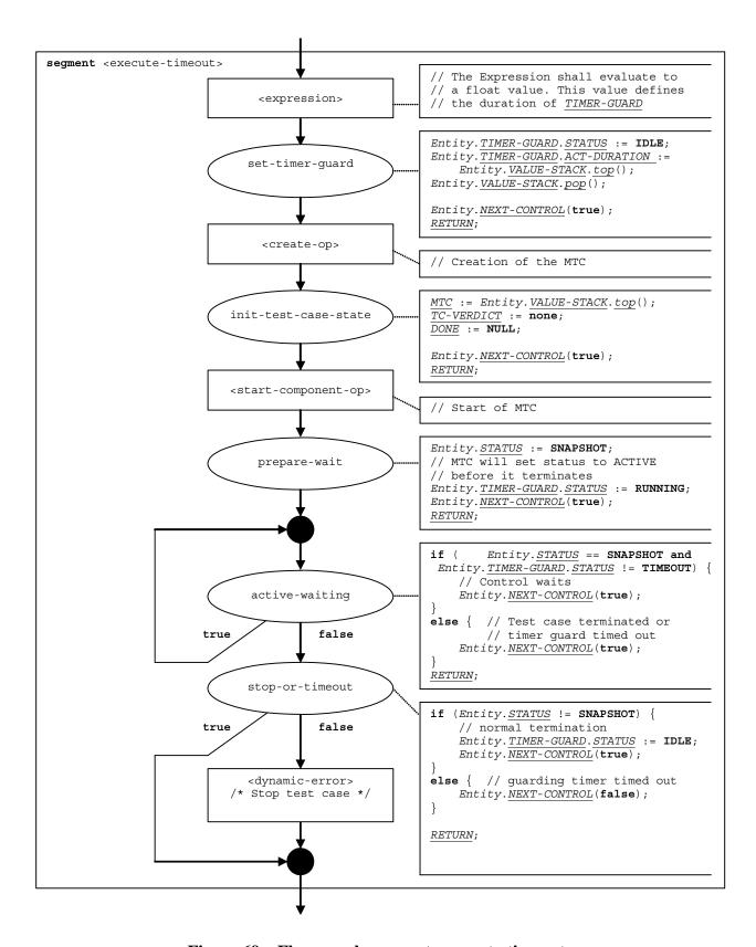
Figure 69 – Flow graph segment <execute-timeout>
