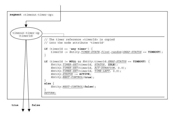
Figure 135 – Flow graph segment <timeout-timer-op>
