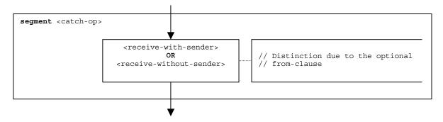
Figure 55 – Flow graph segment <catch-op>
