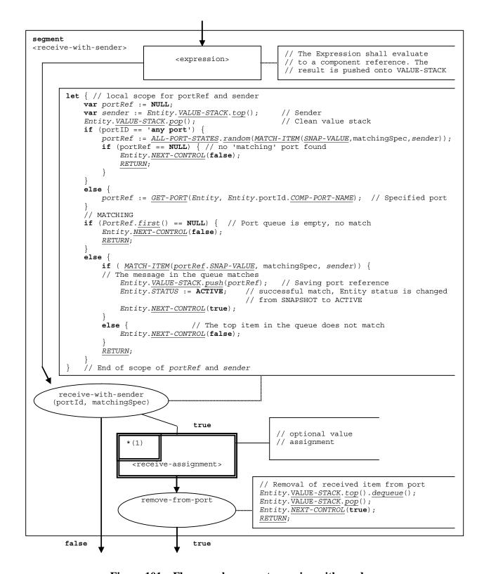
Figure 101 – Flow graph segment < receive-with-sender >
