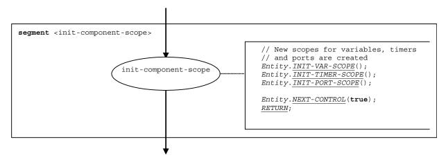
Figure 76 – Flow graph segment <init-component-scope>
