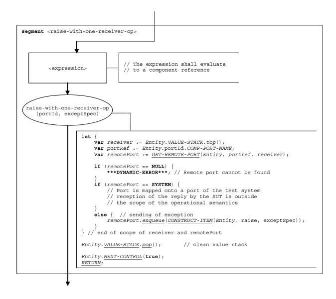
Figure 97 – Flow graph segment <raise-with-one-receiver-op>
