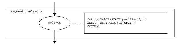
Figure 115 – Flow graph segment <self-op>
