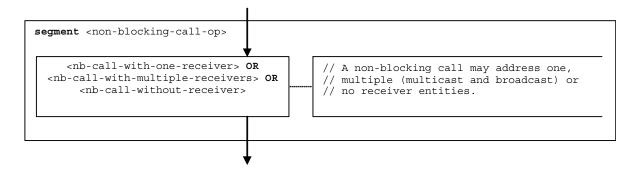
Figure 48 – Flow graph segment <non-blocking-call-op>
