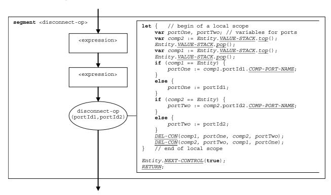
Figure 64 – Flow graph segment < disconnect-op>
