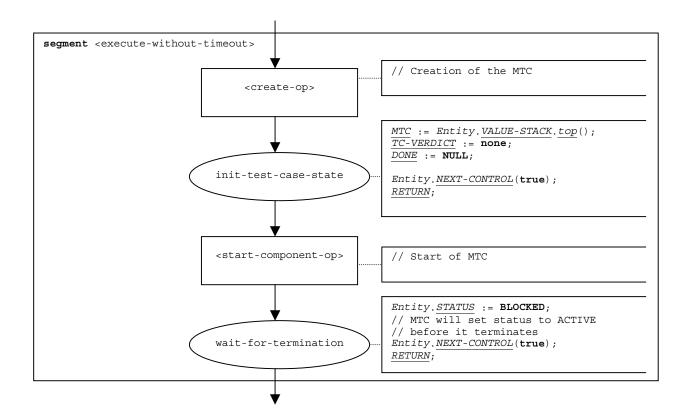
Figure 68 – Flow graph segment < execute-without-timeout>
