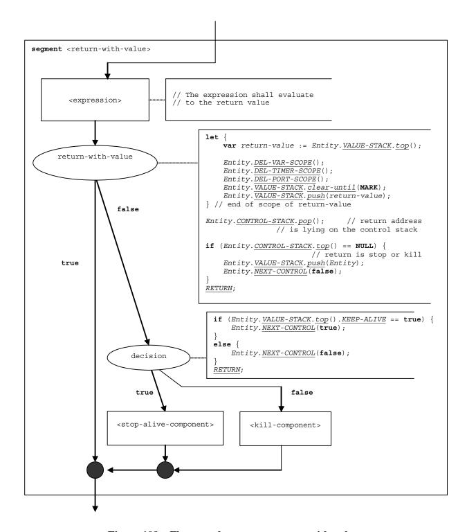
Figure 109 – Flow graph segment < return-with-value>
