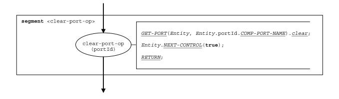
Figure 59 – Flow graph segment <clear-port-op>
