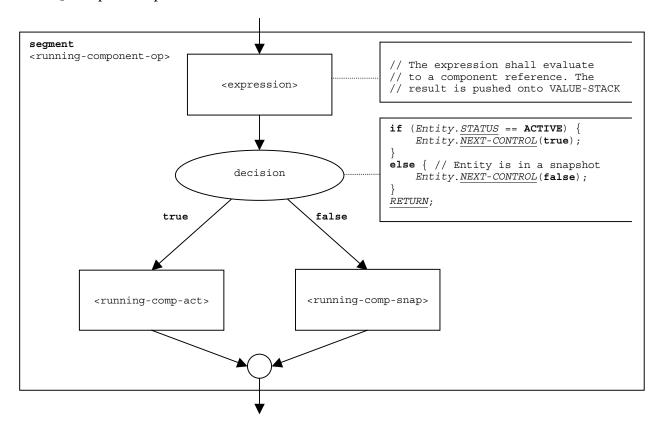
Figure 111 – Flow graph segment <running-component-op>
