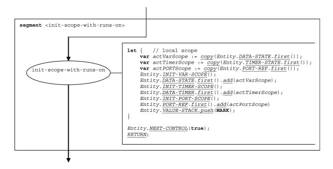
Figure 76-a – Flow graph segment <init-scope-with-runs-on>
