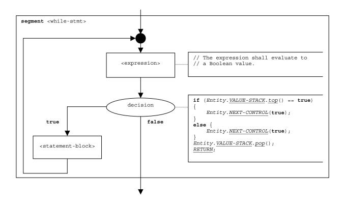
Figure 140 – Flow graph segment <while-stmt>
