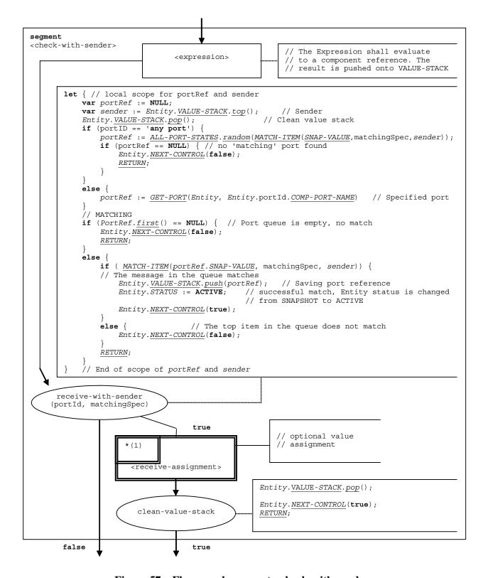
Figure 57 – Flow graph segment <check-with-sender>
