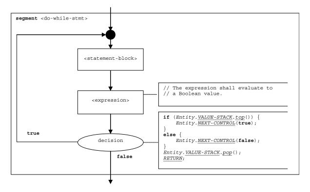
Figure 65 – Flow graph segment <do-while-stmt>
