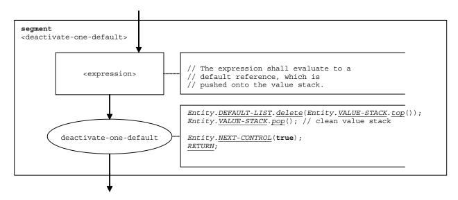
Figure 63-b – Flow graph segment <deactivate-one-default>
