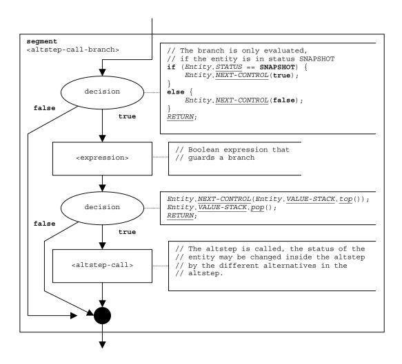
Figure 41 – Flow graph segment <altstep-call-branch>
