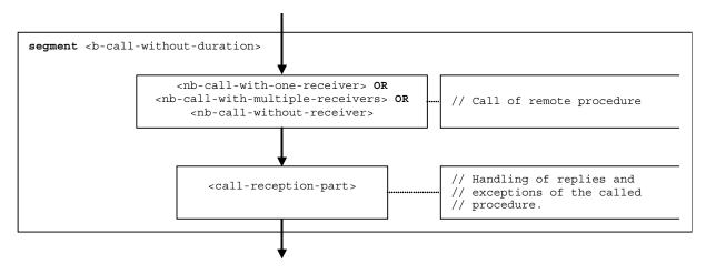
Figure 51 – Flow graph segment <b-call-without-duration>
