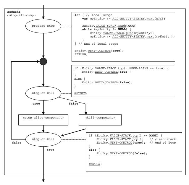
Figure 127 – Flow graph segment <stop-all-comp>
