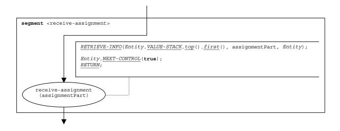
Figure 103 – Flow graph segment < receive-assignment>
