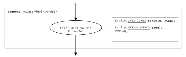
Figure 134 - Flow graph segment < timer-decl-no-def>
