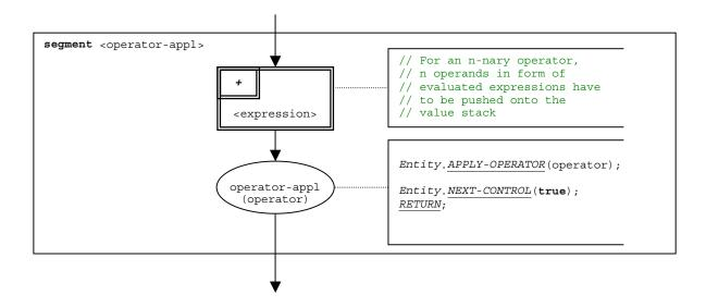
Figure 74-a – Flow graph segment < operator-appl>
