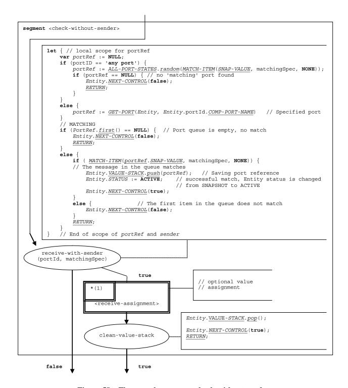
Figure 58 – Flow graph segment <check-without-sender>
