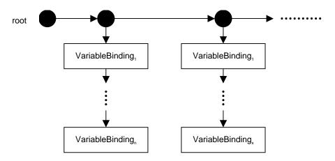
Figure 25 – Structure of the <u>DATA-STATE</u> part of an entity state
