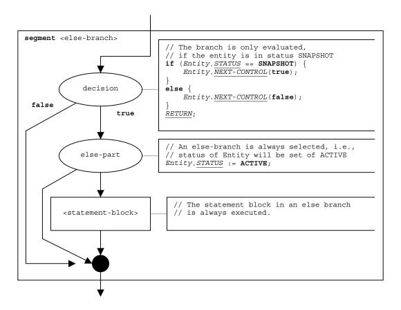
Figure 42 – Flow graph segment <else-branch>
