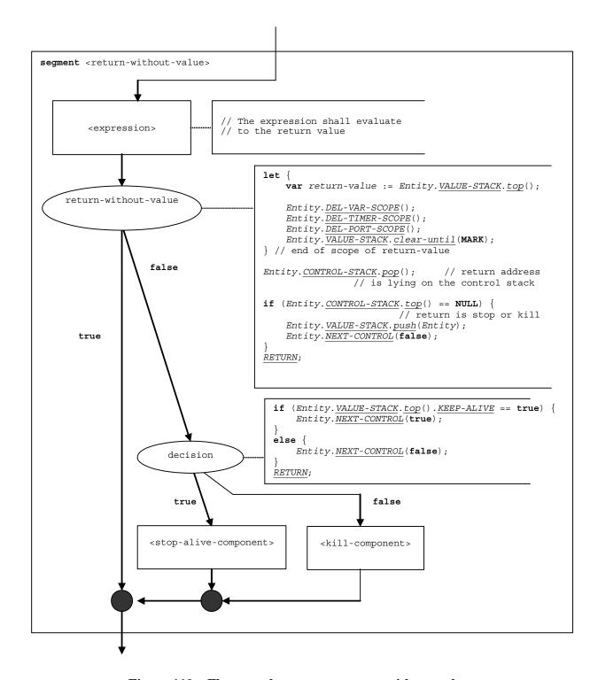
Figure 110 – Flow graph segment < return-without-value>
