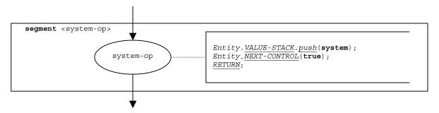
Figure 131 – Flow graph segment <system-op>
