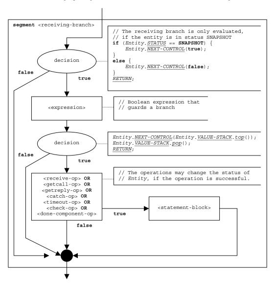
Figure 40 – Flow graph segment < receiving-branch>
