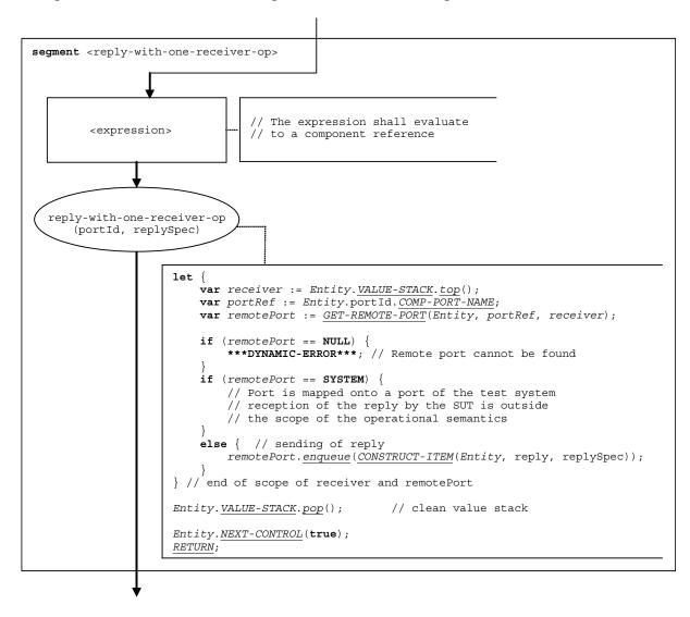
Figure 106 - Flow graph segment < reply-with-one-receiver-op>
