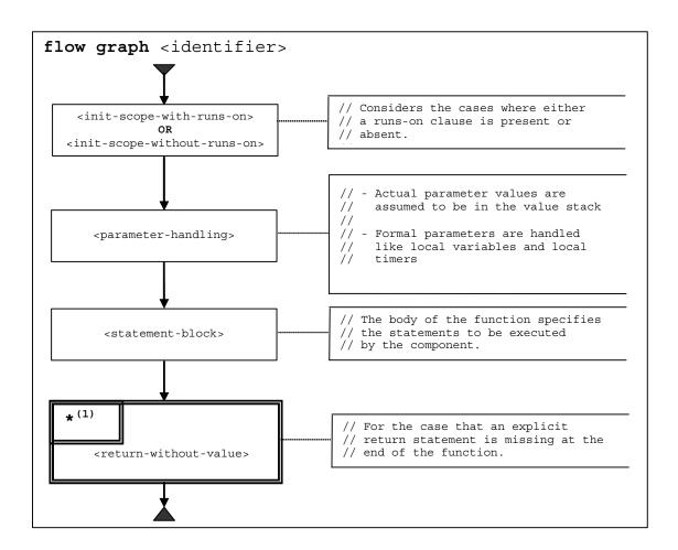
Figure 20 – Flow graph representation of functions
