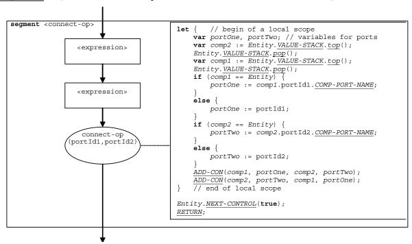
Figure 60 – Flow graph segment <connect-op>
