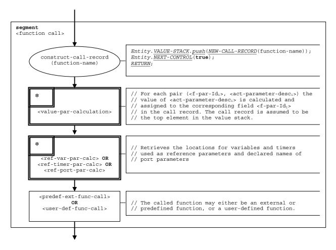
Figure 80 – Flow graph segment <function-call>
