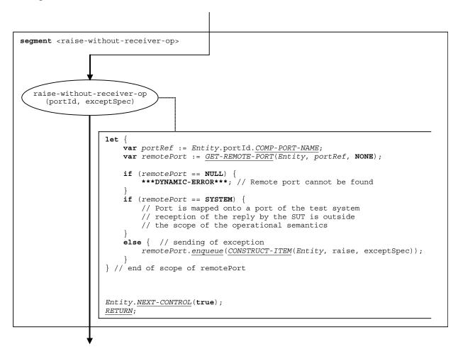
Figure 98 – Flow graph segment <raise-without-receiver-op>
