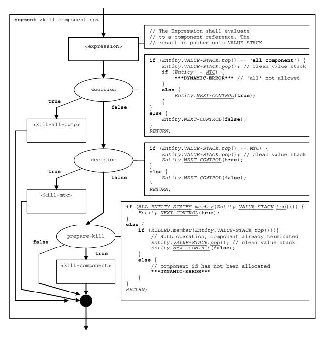
Figure 90-a – Flow graph segment <kill-component-op>
