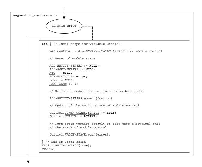
Figure 74-b – Flow graph segment <dynamic-error>
