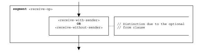
Figure 100 – Flow graph segment <receive-op>
