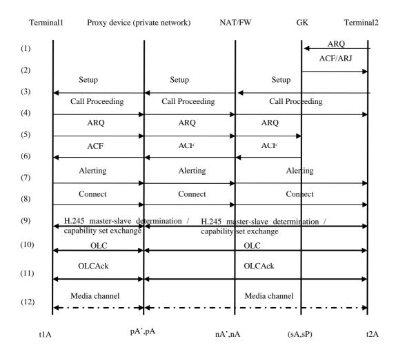
$NOTE-The\ prefixes\ t,\ n,\ p,\ s\ denote\ terminal,\ NAT,\ proxy\ and\ gatekeeper,\ respectively.\ A\ and\ P\ represent\ the\ IP\ address\ and\ the\ UDP/TCP/other\ port\ of\ each\ entity.$
