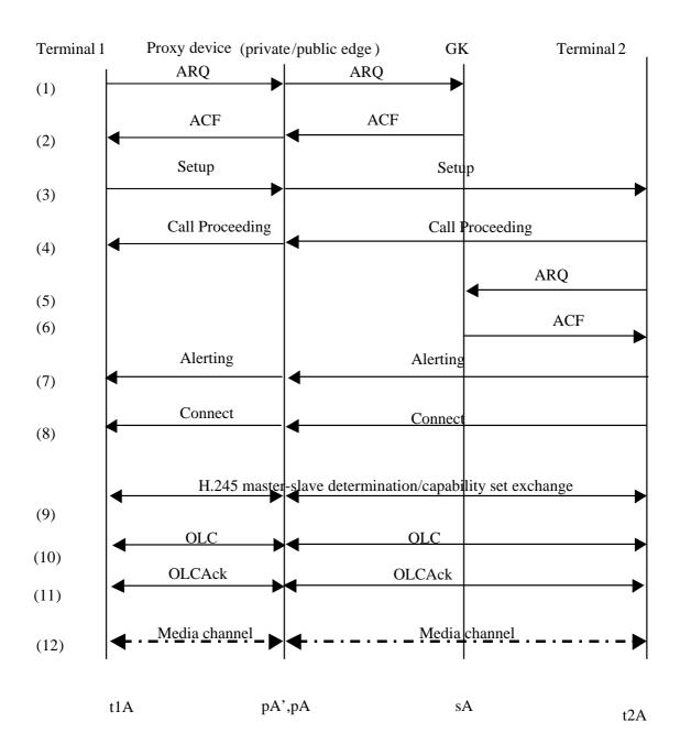
$NOTE-The\ prefixes\ t,\ p,\ s$  denote terminal, proxy and gatekeeper, respectively. A and P represent the IP address and the UDP/TCP/other port of each entity.
