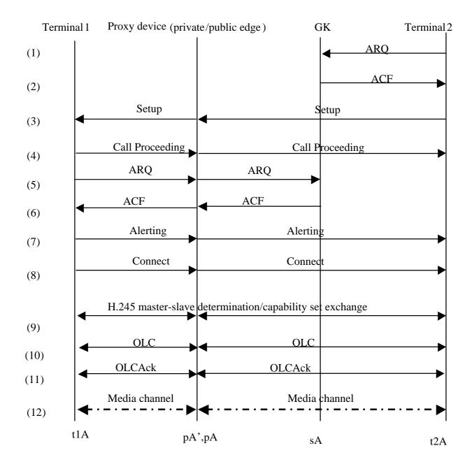
NOTE – The prefixes t, p, s denote terminal, proxy and gatekeeper, respectively. A and P represent the IP address and the UDP/TCP/other port of each entity.
