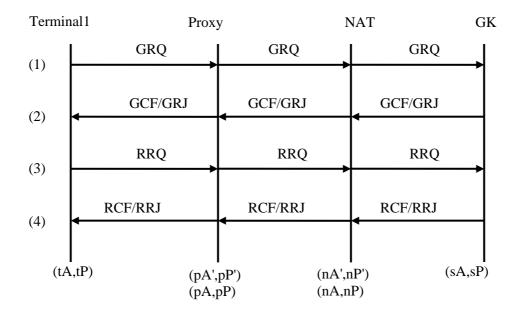
NOTE – The prefixes t, n, p, s denote terminal, NAT, proxy and gatekeeper, respectively. A and P represent the IP address and the UDP/TCP/other port of each entity.
