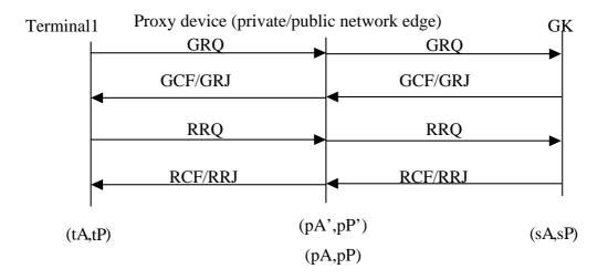
$NOTE-The\ prefixes\ t,\ p,\ s$  denote terminal, proxy and gatekeeper, respectively. A and P represent the IP address and the UDP/TCP/other port of each entity.
